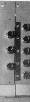
Photograph 1. Suggested front panel construction for the graphics system TTL level outputs. The left-hand 19-inch panel holds the I (monochrome), SYNC, and SYNC output sockets, the right-hand panel holds outputs R, G, B, and I for full colour applications.
